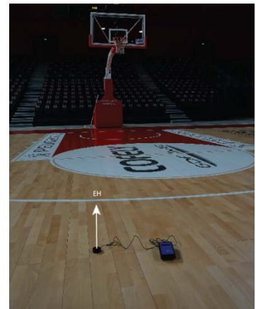
Horizontal illuminance (EH) measurement
