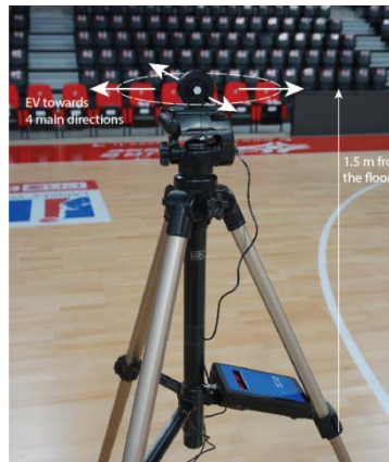
Vertical illuminance (EV) measurement
